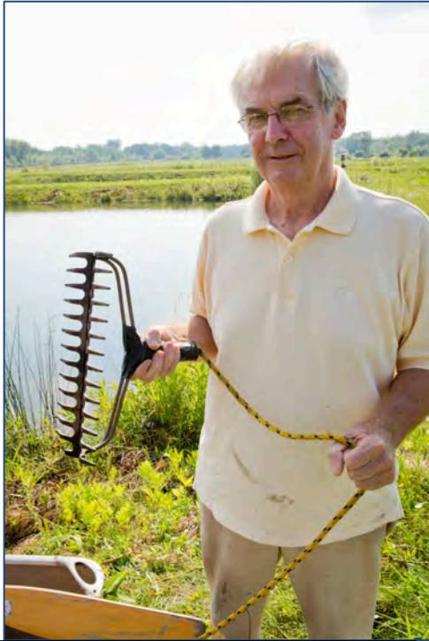
Bob Johnson of Racine-Johnson Associates, Ithaca NY, holds a lake rake used in rake toss surveying.
