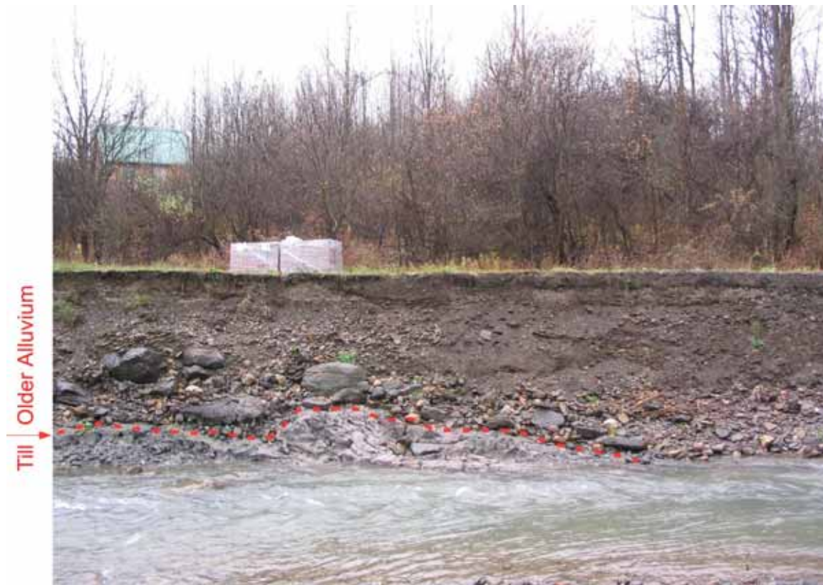
Figure 12. Cutbank with thick deposit of older (300-400yrs b.p.) alluvium overlying till just upstream from German Crossroad.
